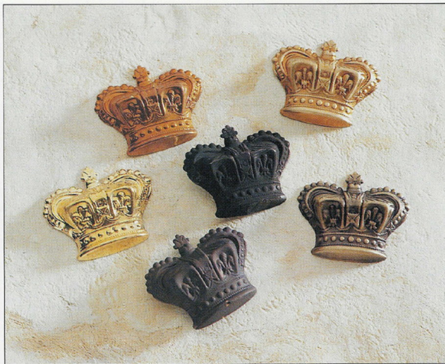
All of these crowns except the 'yellow' one on the far left were immersed for various lengths of time in a selenium-based conversion coating. Then, the two on the far right were mechanically finished and clear-lacquered to remove the excess antiqing agent and bring out the highlights. These samples were prepared by Eric Olander of EPI in New Berlin, WI, a supplier of metal-finishing chemicals.
