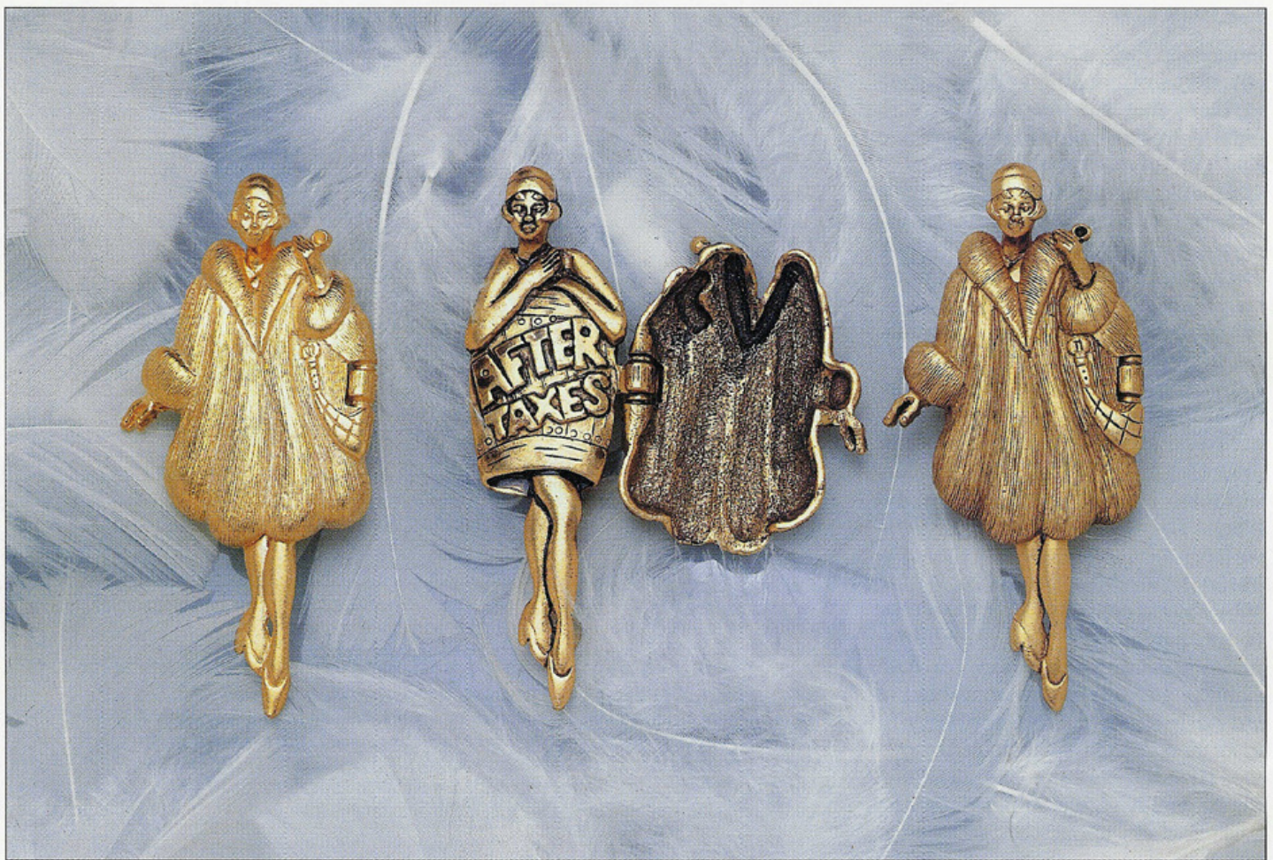
The three stages of producing an antique finish in jewelry using non-conversion coating (l to r): First, the part is plated. Second, it is dipped in a black lacquer. Third, the part with black lacquer is 'relieved' using hardwood peg media in an oblique tumbling barrel. The jewelry designs and highlighting were done by Alan Jewelry (a Danecraft company) in Providence.
