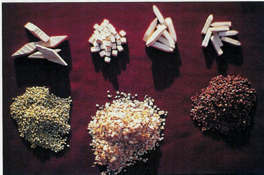
Various types of dry media used in 'dry' relieving: Pre-formed hardwood media are shown across the top, while corncob granules, sawdust flakes and walnut-shell granules are on the bottom. The media are supplied by PEGCO Process Laboratories in Bartlett, NH.
