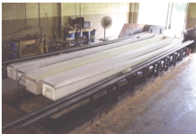
A top view of a custom made 30 foot long, 5-tank system for the InstaBlak process. This shows the versatility of the room temperature process as economical small volume tanks can be constructed to blacken extra long parts.
