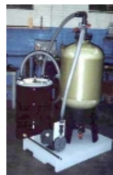
In those rare instances where local regulations require treatment of the rinse waters before discharging them to the sewer, EPI has an ion exchange unit available to add to the system for zero discharge of metals.
