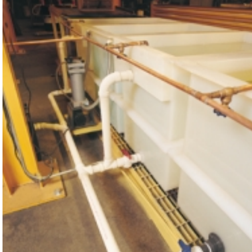
Backside view showing the rinse water inlet pipes and the overflow pipes for the rinse tank, to the drain pipe. Also shows the filter for InstaBlak® 333 solution.
