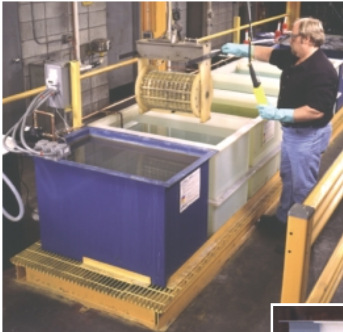
An operator is blackening small parts in a slowly rotating acid resistant plastic barrel. The barrel is moved through the line from tank to tank, using an overhead manual hoist.
