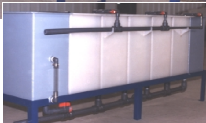
A rear view of the tank system showing the plumbing for the water inlets to the overflowing rinse water tanks and the plumbing outlet pipes from the overflowing rinses along the bottom. Also shown is the vertical glass or clear plastic pipe used as a sight gauge to measure the volume of water displaced to the bottom of the tank by the water displacing E-Tec rust preventive. The water is periodically drained off.
