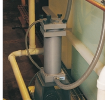
View of a tank system showing the filter used to filter the white by-product precipitate from the InstaBlak 333 solution. By continuously circulating the solution through the filter to remove this white precipitate, it extends the life of the blackening solution.
