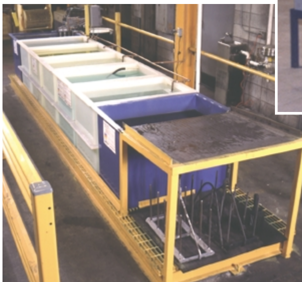
An end view of a seven tank system showing the final steel E-Tec tank and the steel drain board attached to the E-Tec tank. Below the drain board are several racks used to hold larger parts to be blackened rather than using a rotating barrel which could not be used because of the size of the parts.
